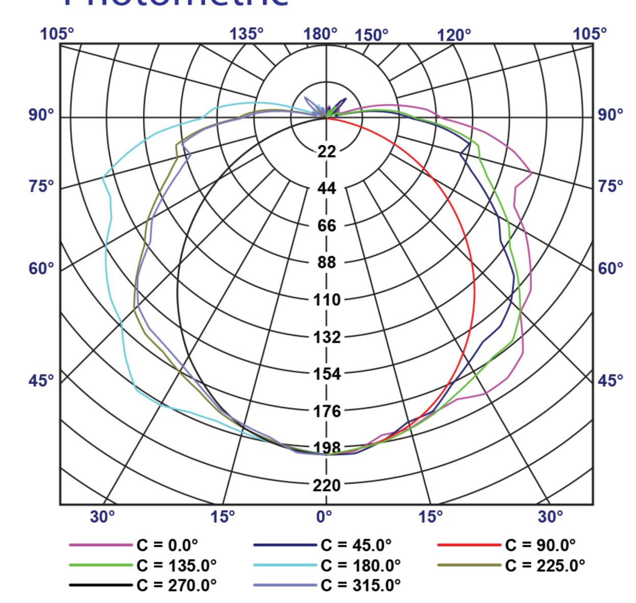
Luminous intensity values are shown radially from centre. Elevation angle values are shown around the outside of the graph. Report No: J20202120498
