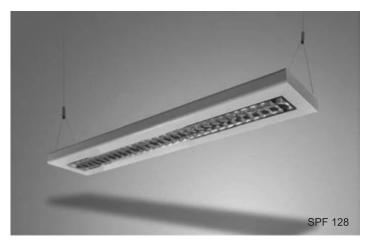
Direct/Indirect Light recessed mounted luminaires for T5 fluorescent Lamp. Limited luminance L  $\leq$  1000 cd/m² of reference angle above 65° all round. Provides comfortable light effect with suspension system for easy alignment and height adjustment. Ideal for offices, school, libraries, and commercial building where VDT terminal and frequently use.
