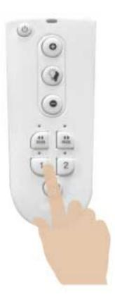
3. To unpair specific lighting units from grouping, place the remote within close range (10cm) for best result and click the red program button and "1-2" until LED indicator starts blinking.
